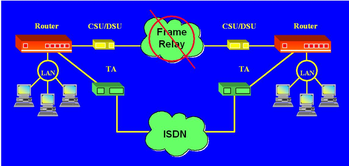
The Terminal Adapter “listens” for data by monitoring the Data Terminal Ready lead in the RS-232 or V.35 interface. This lead, or wire, only becomes energized when the router attempts to send data over the secondary path.
